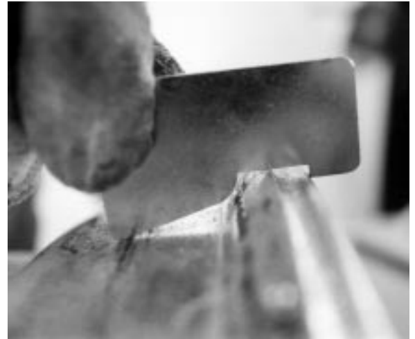
Photo 1. Acceptable Rim Flange Wear Condition
