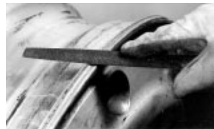
Photo 4. Removing sharp edge by hand with a metal file.
